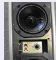
Connection bay with cover removed.
